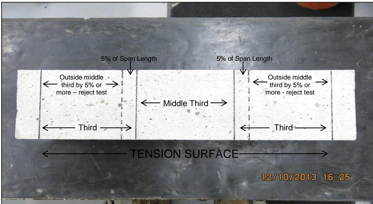
1. If the fracture initiates in the tension surface within the middle third of the span length and the testing machine supplies modulus of rupture (R), record results per the REPORT section.
