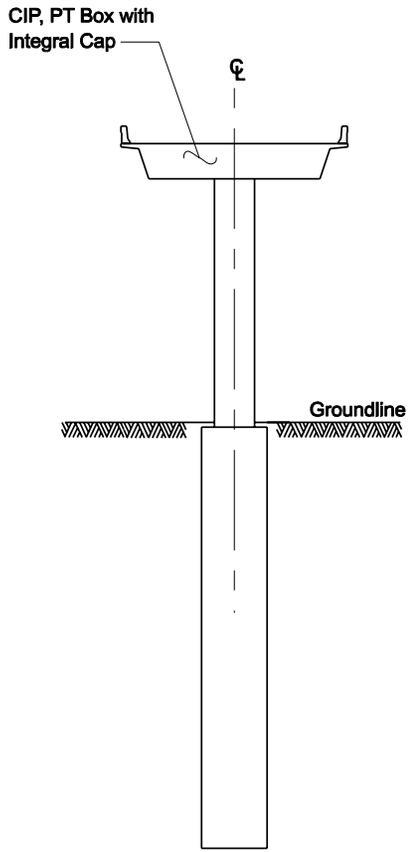
**SINGLE-COLUMN PIER WITH DRILLED SHAFT**
