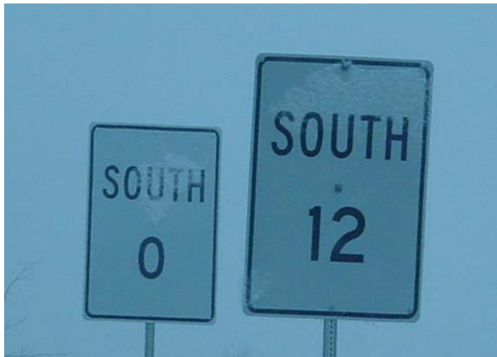
Figure 3-2. Illustrates Very Little Difference in Snow Accretion and Tilt (Storm date 12-29 & 30-2004)
