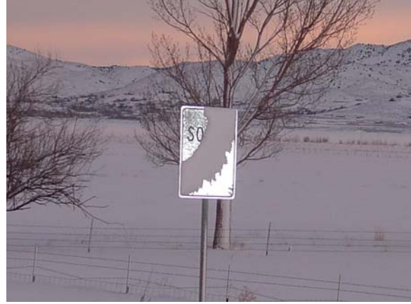
Figure 3-5. Illustrates Inconsistent Pattern of Snow Accretion (Storm date 1-11-2005)
