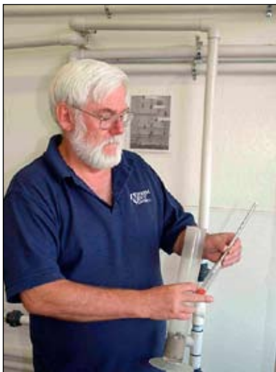
Maintenance Supervisor Tom Lumpkin tests salt content of brine.
