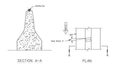
BARRIER RAIL REFLECTOR INSTALLATION
