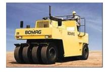
Figure 6-203.3. Pneumatic Tired Roller.
