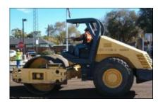
Figure 6-203.1. Steel Wheel Vibratory Roller.
