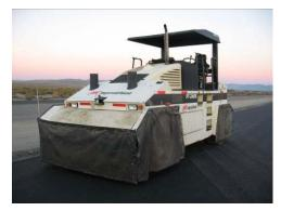
Figure 6-401.7. Rubber Tired Pneumatic Roller with Skirting.
