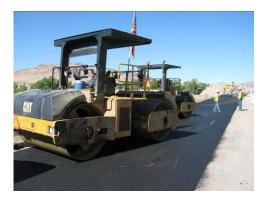
Figure 6-401.6. Steel Wheel Roller.
