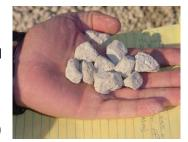
Figure 6-401.2. Aggregate Properly Coated with Lime.
