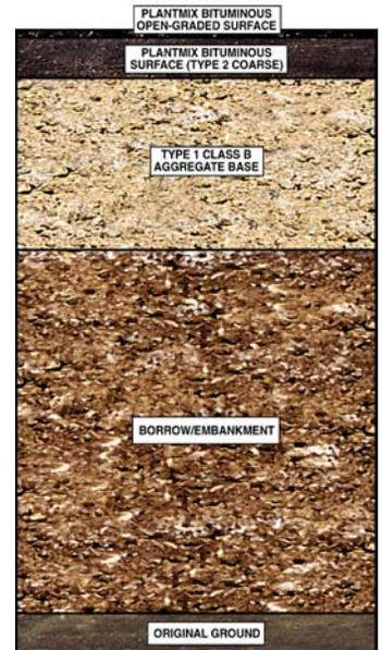
Figure 6-300.1. Typical Roadway Structural Section.
